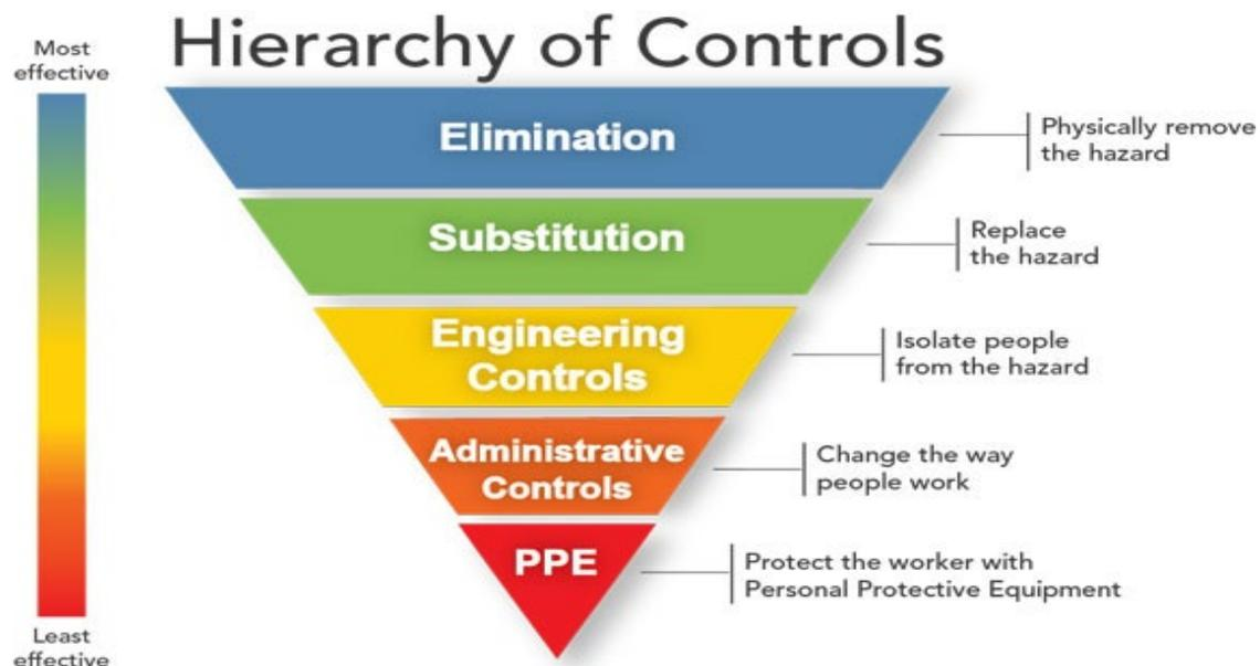
The chart identifies the preferred way to control a hazard from the most effective which is elimination. Then the order follows the next preferred method using Substitution, then Engineering Controls, Administrative Controls then the least effective, Personal Protective Equipment (PPE).
